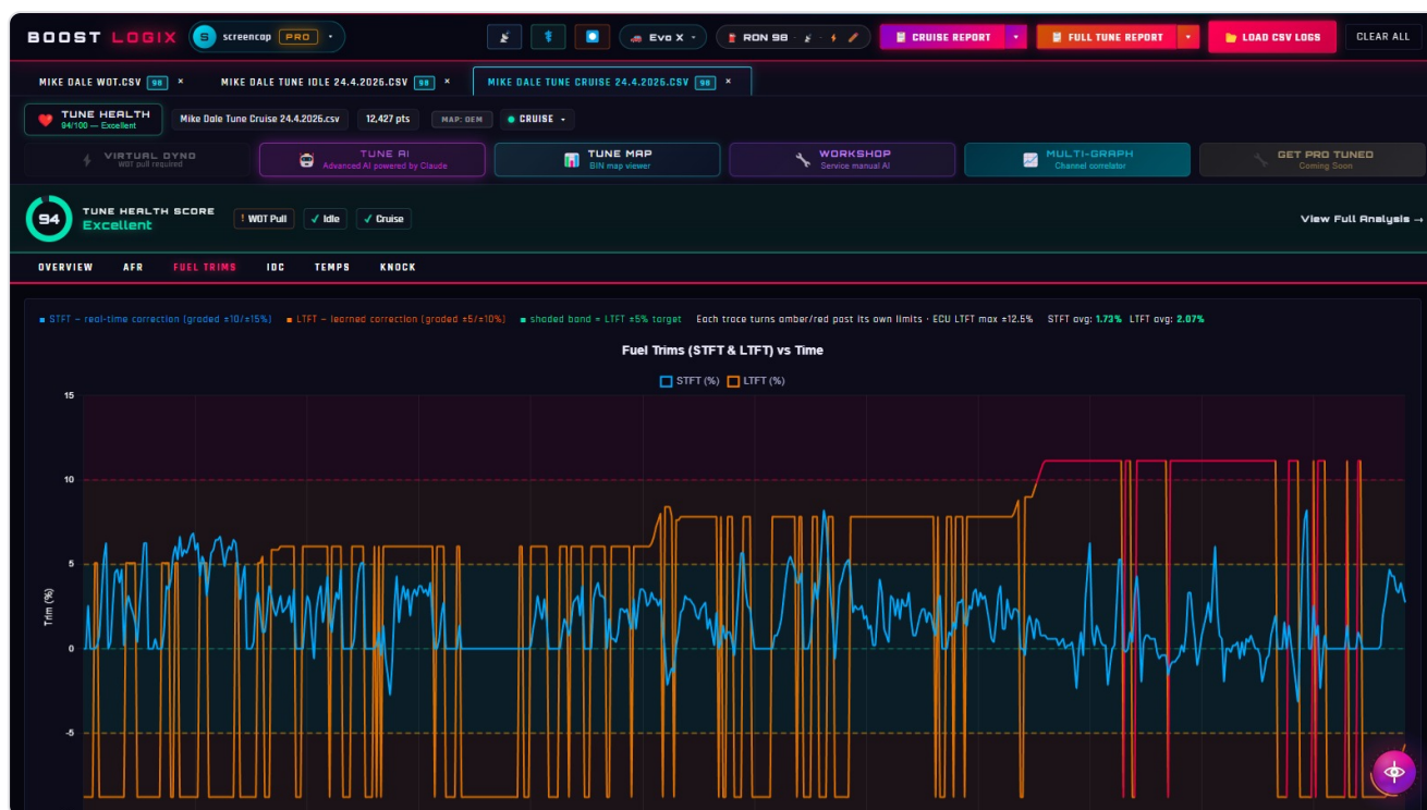
The Fuel Trims tab on a cruise log showing LTFT and STFT
