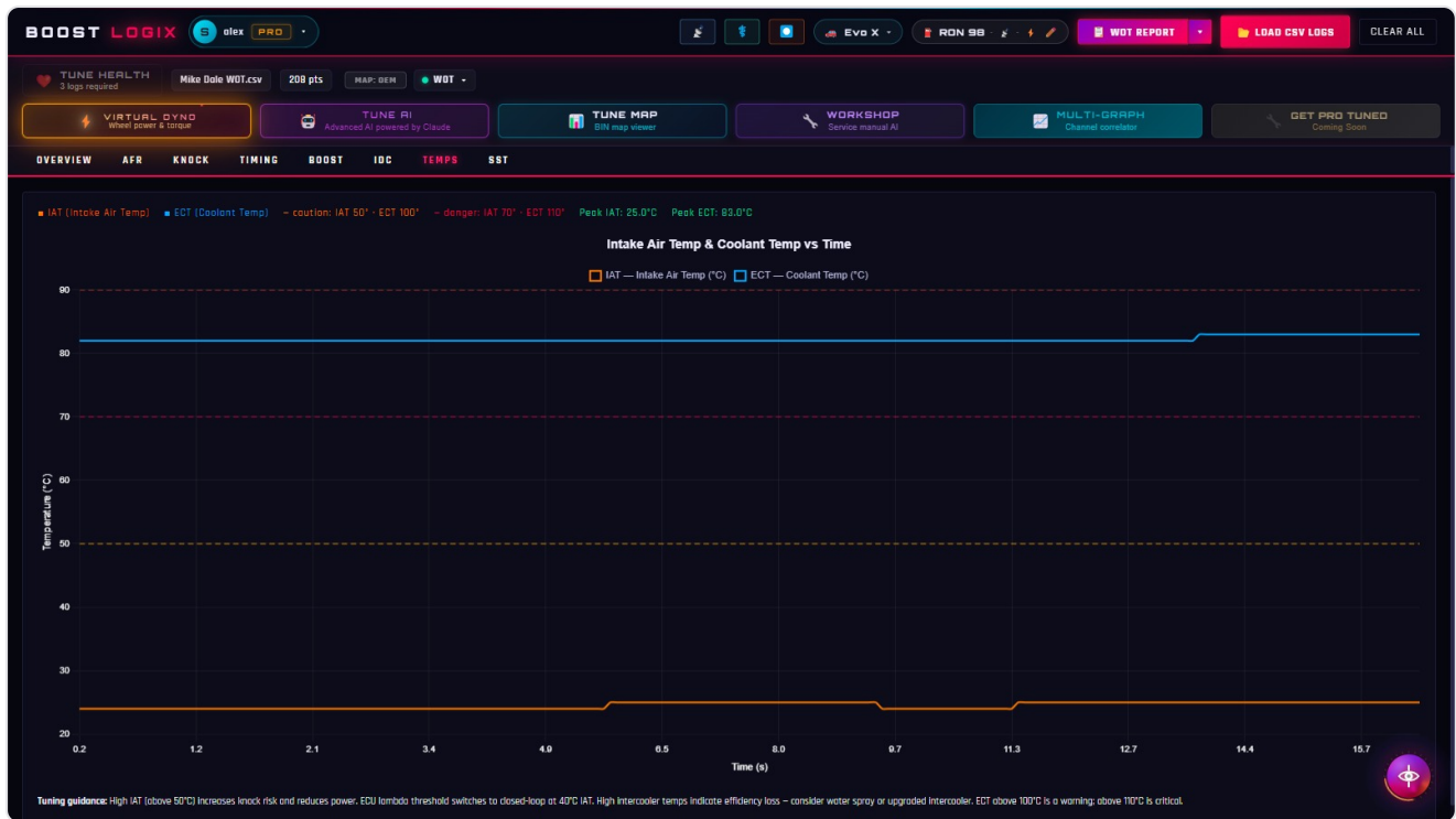
The Temps tab showing ECT, IAT and MAT traces with limit lines
