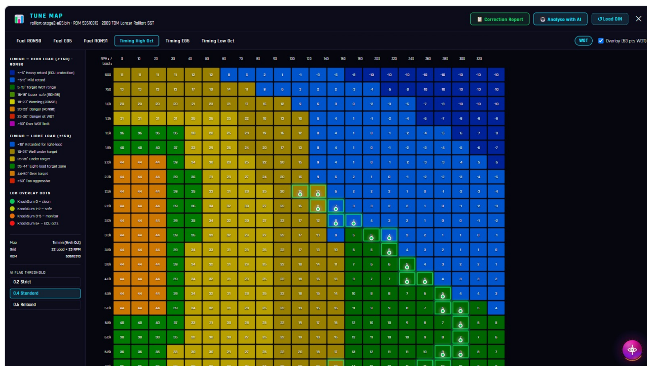
A timing map with log overlay dots and the log-type pills
