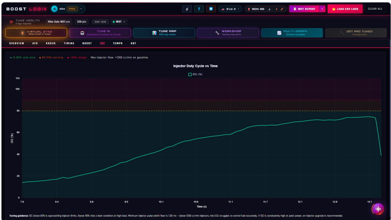
The IDC tab showing injector duty cycle under boost
