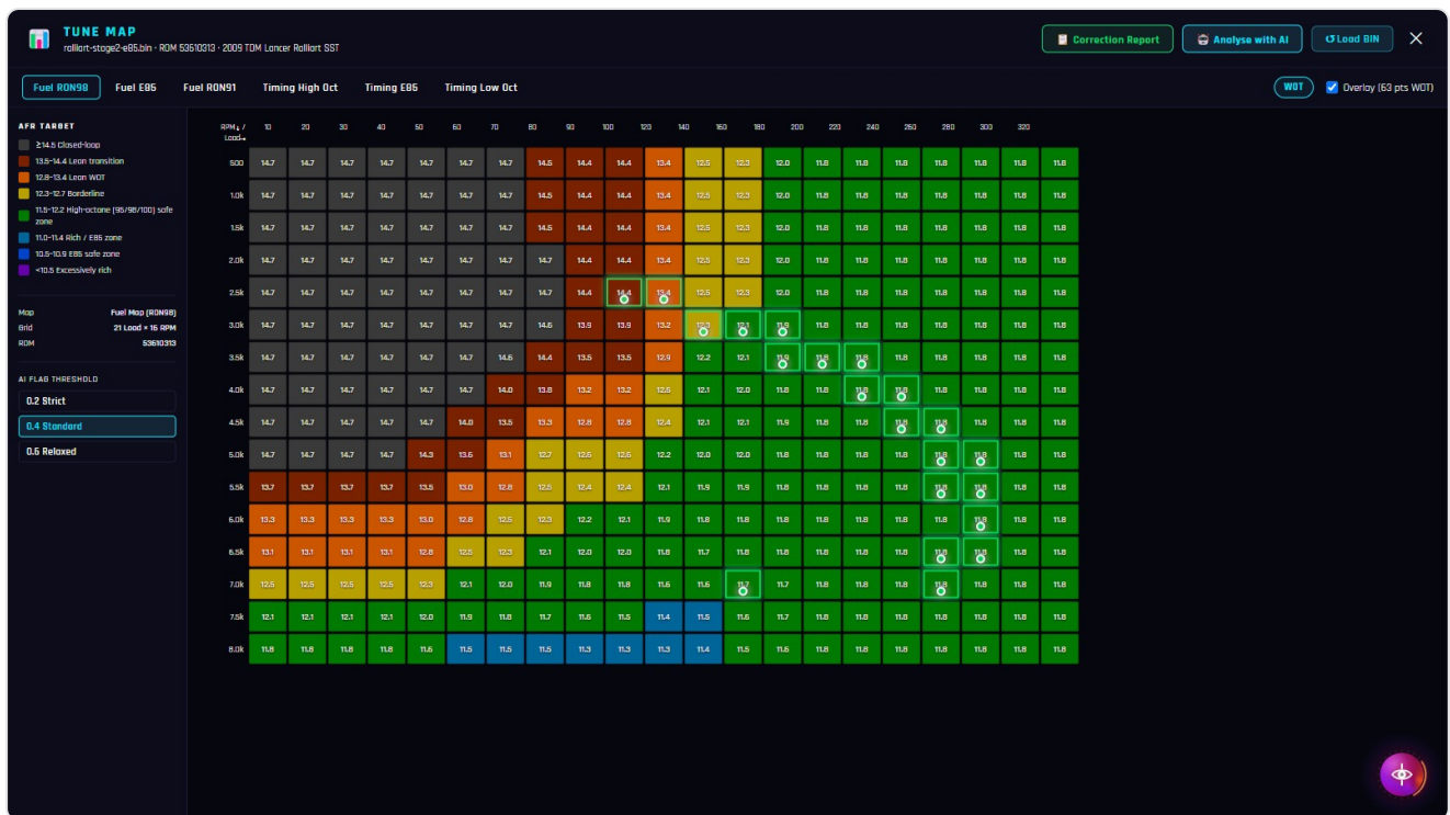
A fuel map shown as a colour-coded heat-map grid
